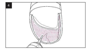
4. Hold the orthosis in your hand with the tip pointing downwards (cap pointing towards the person) Apply the adhesive only to the entire cap (ascending from cap tip to cap end).
