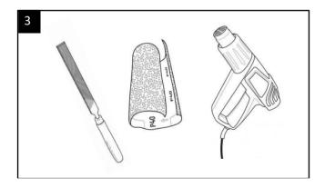
3. Roughen the claw wall with a rasp and the orthosis with the sandpaper in the cap. If necessary dry both with a hot air gun.
